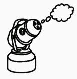
Apply **BIOBUBBLE COAT 90D** over the pre-cleaned surfaces with an Electrostatic Fogger.
